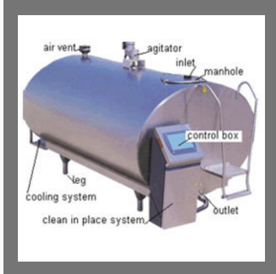
Horizontal Milk Storage Tank
